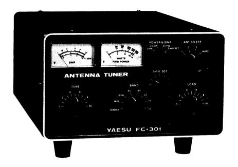
The FC-301 antenna coupler is designed for low and medium power applications in the HF amateur bands from 160 through 10 meters. It is designed to minimize the adverse effects of high SWR on a coaxial line or wire antenna which may result in difficulty in tuning a transmitter designed to work into a resistive 50 ohm load.
